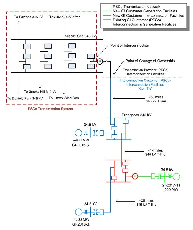
Figure 2: GI-2017-11 Interconnection to 345 kV Bus in Missile Site Substation
